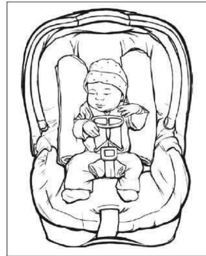
Figure 1: Car safety seat with a small cloth between the crotch strap and infant; retainer clip positioned at the center of the chest, level to the infant's armpits; and blanket rolls on both sides of the infant.
